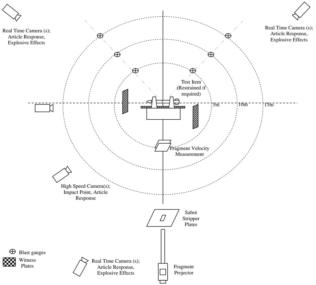
**Figure 17.14.2: TYPICAL SETUP FOR 1.6 ARTICLE FRAGMENT IMPACT TEST**
